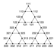
all three disks start on peg 1, then they can be moved to peg 2 in seven moves by following the sequence down the right side of the triangle.
